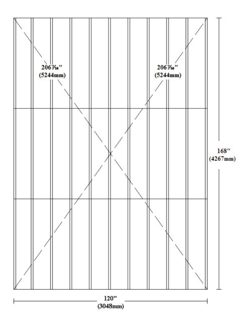
NB:- Floor joists run from gable to gable.
